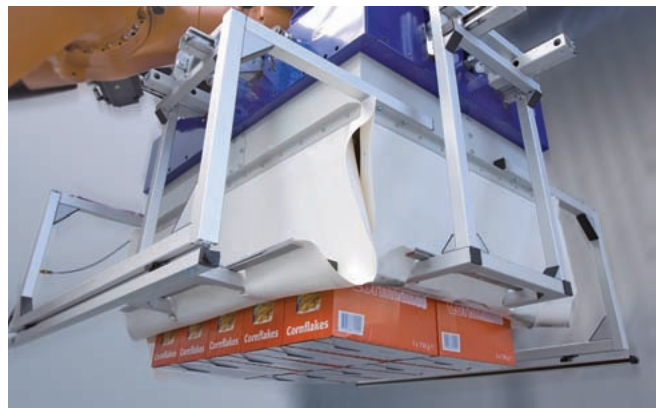
Vacuum layer gripping system SPZ for handling of cardboard boxes
