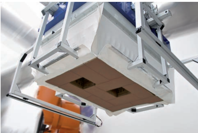
Layer gripping system SPZ with mechanical clamping and skirt
