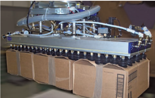
Large-area vacuum gripping system FXC-SG for handling of bending cardboard boxes
