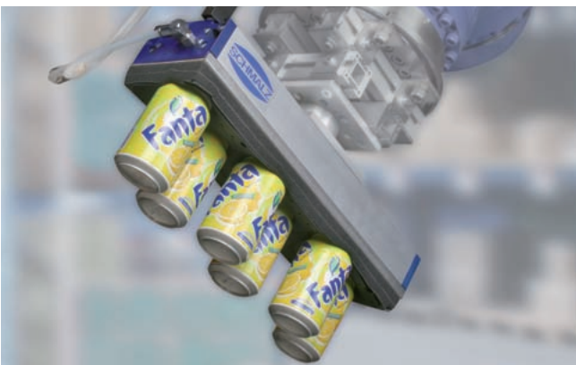
Large-area vacuum gripping system FXC with combifoam for handling of cans
