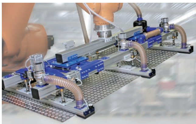
Vacuum suction spider SSP-FMC for handling of checker plates
