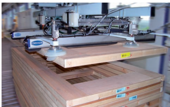
Large-area vacuum gripping system FXC for handling of doors
