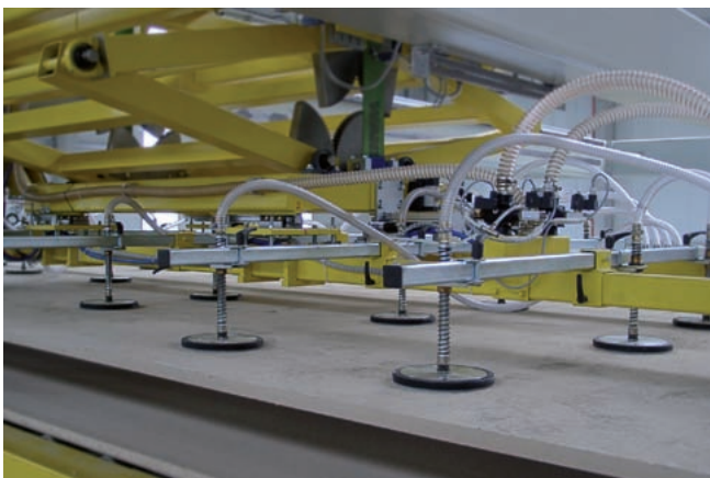
Vacuum suction spider SSP with suction plates
