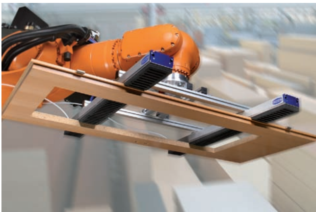
Large-area vacuum gripping system FXC/FMC for handling of doors
