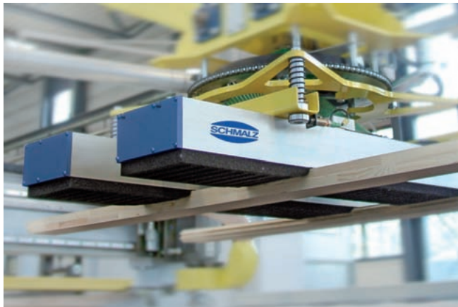
Large-area vacuum gripping system SBX for handling of wooden boards
