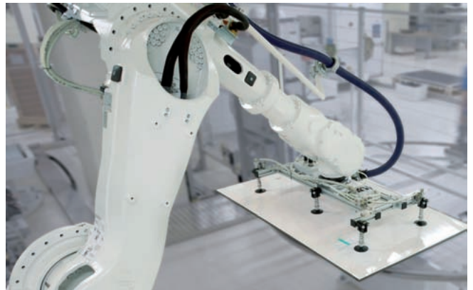
Solar industry: vacuum suction spider SSP for handling of solar modules
