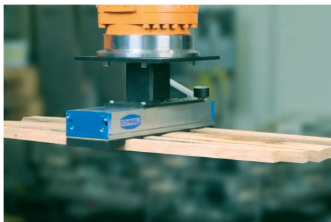
Large-area vacuum gripping system FXC for powerful handling of wooden boards
